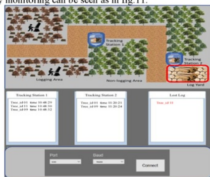
Fig.11: Interface Monitoring System Log at Log Yard
