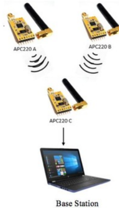
Fig. 2: Wireless Sensor Network Topology Using APC220
