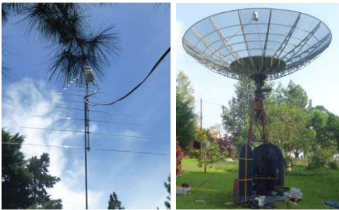
Figure 6. Antenna for radio telescope receiver, LPDA for continuum observation (left), parabolic antenna for spectral observation (right)
