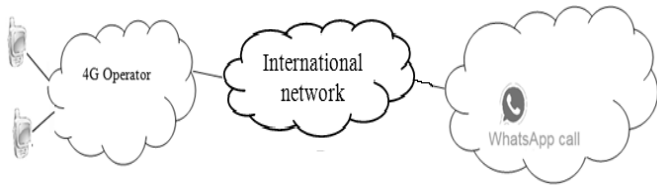
Fig. 3. WhatsApp Call topology on 4G mobile network.
