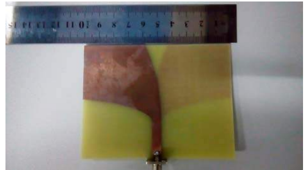
(a) front view of realized single antipodal Vivaldi printed antenna
