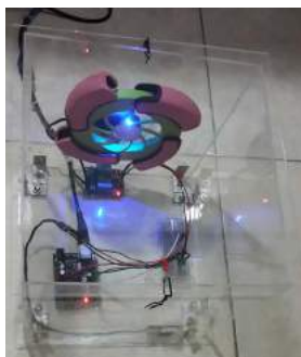
Figure 7. Control System Room Temperature
